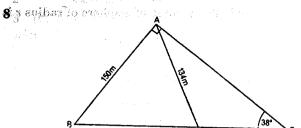
The diagram represents a triangular plot of ground ABC, situated at the junction of two straight roads BA and BC. Under a road-widening plan the section ABP is cut off. Given that BA = 150 m, AP = 134 m,  $A\hat{C}B = 38^{\circ}$  and  $B\hat{A}C = 90^{\circ}$ , calculate
