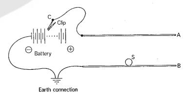
The diagram shows a section through two horizontal metal plates A and B; B is earthed, and A can be given a potential V by using the movable clip C to connect it to a terminal on a high-voltage battery. S is a small sphere of conducting material, resting on B.
