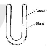
The diagram illustrates a double-walled vacuum flask used for keeping its contents hot.
