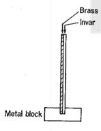
The compound bar of brass and invar shown in the diagram is firmly secured to a metal block at its lower end.
