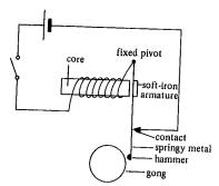
The diagram shows the essential features of a bell operated by a battery. Explain why the hammer repeatedly strikes the gong after the switch has been closed. [5]
