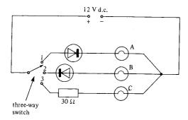
Without carrying out any calculations, state and explain whether each lamp will light brightly, dimly or not at all when the three-way switch is moved successively into positions 1, 2 and 3.
