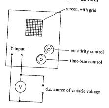
The diagram shows some of the essential features of a cathode-ray oscilloscope (c.r.o.) with a variable source of d.c. voltage connected to the Y-plate terminals. The time-base control was set so that a horizontal line appeared across the face of the screen.
